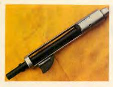
ABOVE: Telescoping bolt and barrel from Beretta Model 12S. Of total barrel length of 7.9 inches, 5.9 inches lie inside bolt-block at moment of firing, reducing muzzle climb to absolute minimum. BELOW: Trigger assembly on Beretta Model 12S shows fireselector switch for Rapid, 1 (semiauto) and Safe.
